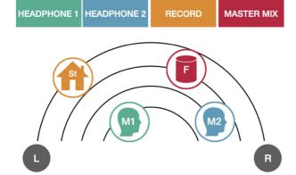
Local mix settings control and monitor the mix of all available signals, such as headset microphones, recordings, any available file playback, the remote end, (e.g. the master control room) to receive instructions and, if available, the local ambience as well. The operator can do the optimal mix for themselves as well as for all other connected headsets, like co-moderators or guest-commentators. Remote control of the local mix is also possible.
